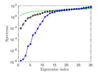
FIG. 5. Spectrum of the matrix W defined in (7) for controls generated by OGRA (green, vertical lines), GRA (black, circles) and for RCC (blue, squares). Dimensionless units are used.
