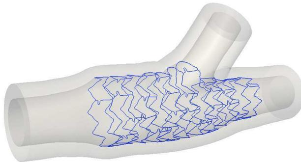
Figure 2: An illustration of a realistic cardiovascular stent implanted into an arterial bifurcation. The stent is depicted by means of its centerline. The length of the visualized portion of artery is about 2 centimeters, while the inner and outer reference diameters are equal to 2.78 and 4.58 millimeters respectively, [16].
