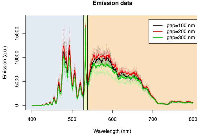
Figure 1: Emission data captured in the factorial laser welding experiment (dashed lines), colored according to the three different gaps; and means of the three groups, corresponding to the three different gaps (solid lines). The figure is divided along the abscissa into the plasma (light blue), laser (light green), and thermal (light red) emissions.
