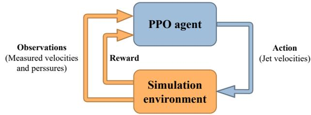
Figure 3: Schematic of the PPO agent closed-loop control.
