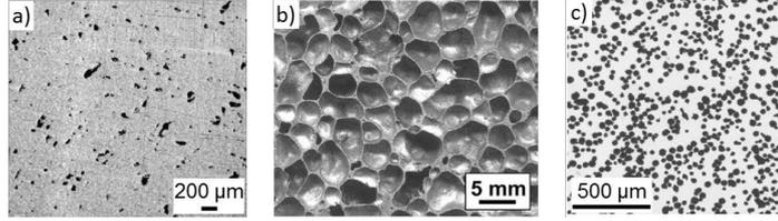
**Figure 1:** Examples of image data for quality monitoring applications: a) pores in products obtained via metal additive manufacturing , b) cross-section of a metal foam , c) micrographs of steel powder particles for metal additive manufacturing
