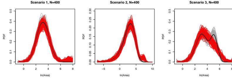
**Figure 4:** Comparison between 100 in-control density curves (grey lines) and 100 out-of-control density curves at the highest severity level (red lines) for different scenarios at  $N = 400$ ; cross-sectional average curves are depicted with solid thick lines.
