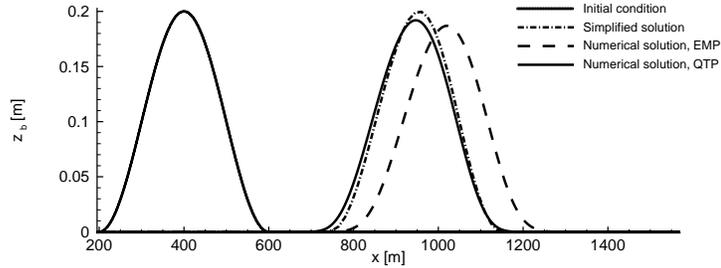
Figure 6: Comparison between the approximate and the numerical solutions in the case b),  $\epsilon = 0.06$ , at time  $t = 30000s$ .
