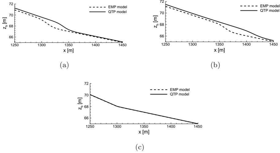
Figure 8: Comparison between the QTP and the EMP model of the bed evolution (time = 450s) in the case a)  $c_0 = 0.002$  and  $\epsilon = 0.003$ , b)  $c_0 = 0.0012$  and  $\epsilon = 0.002$ , c)  $c_0 = 0.00012$  and  $\epsilon = 0.0002$
