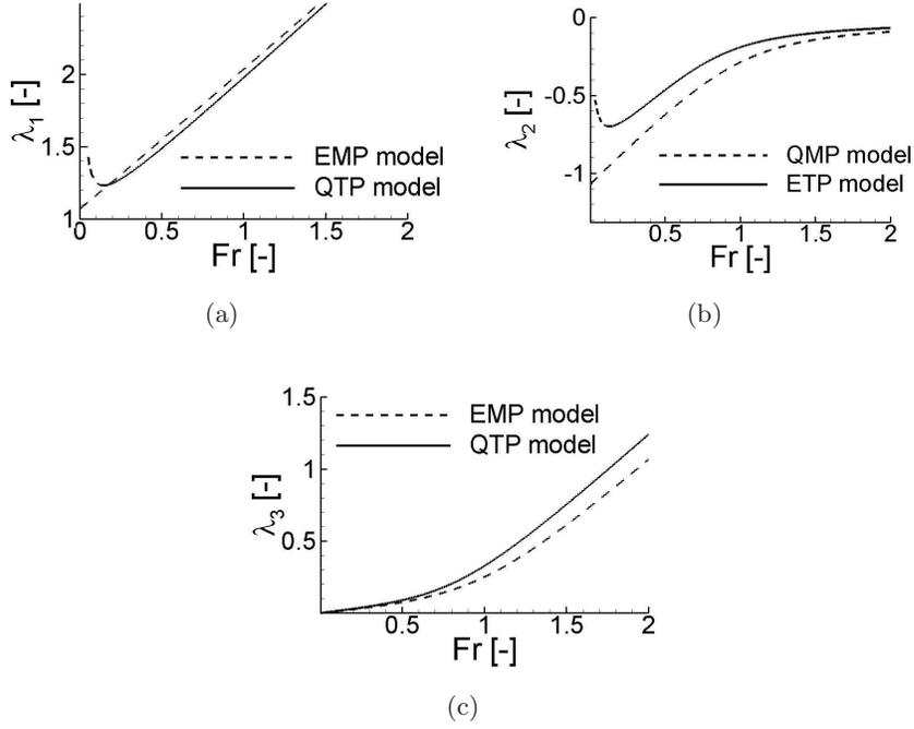
Figure 4: Comparison between the QTP and the EMP system eigenvalues with  $c_0 = 0.03$ .
