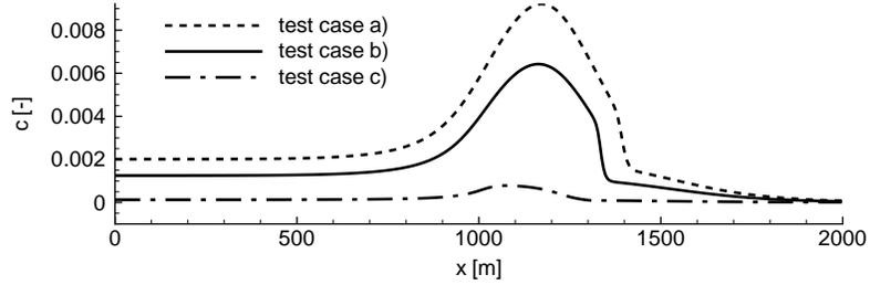
Figure 9: Solid concentration at the time 450s for the three test cases.
