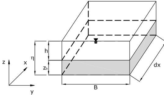
Figure 1: Control volumes for determination of shallow water equations with mobile-bed.
