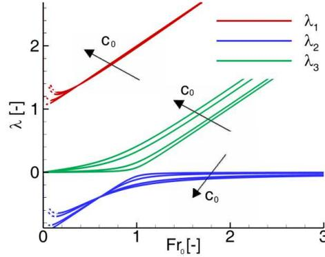
Figure 3: Eigenvalues for the QTP system. Sediment concentration  $c_0$  increasing from 0.000002 to 0.045. The lines are dashed for small values of the Froude number, because high concentrations with small Froude number are not physically meaningful.
