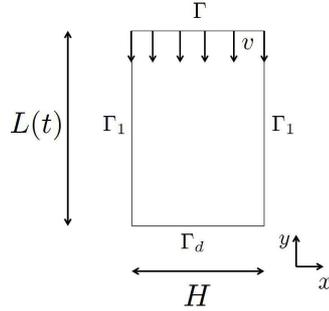
Figure 4: Movement of domain  $\Omega_c$ . The velocity of the boundary is  $\mathbf{w} = -v\mathbf{j}$ ,  $\mathbf{j}$  being the unit vector of the  $y$  axis. Thus, the length of the slab is  $L(t) = L_c - vt$ , while the width,  $H$ , is fixed.
