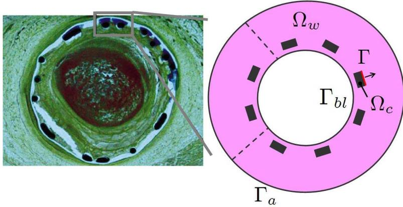
Figure 1: Section of the artery with the implanted stent on the left. Schematic representation of the two dimensional computational domain on the right. The dark areas represent stent elements, the  $\Omega_c$  domains. The mass transport takes place through the boundary  $\Gamma$ . The remaining colored region represents the tissue,  $\Omega_w$ .
