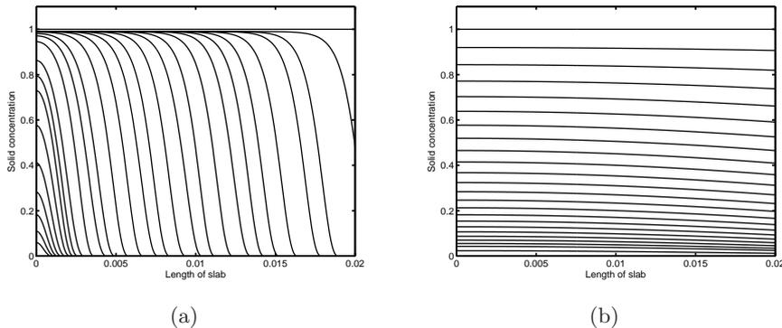
Figure 5: Solid drug profiles in  $x = H/2$  at different values. The initial concentration is  $s_0 = s(\mathbf{x}, 0) = 1$ . In (a) the case of  $\delta \gg 1$ . The matrix divided in two distinct regions and the dissolution front progressively moves inside the matrix. In (b) the case of  $\delta < 1$ . The solid concentration decreases uniformly in time.
