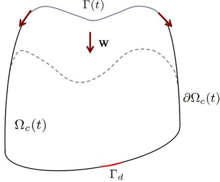
Figure 2: Schematization of the surface erosion problem. The moving boundary  $\Gamma(t)$  slides on  $\partial\Omega_c \setminus \Gamma(t)$  with velocity  $\mathbf{w}$ .
