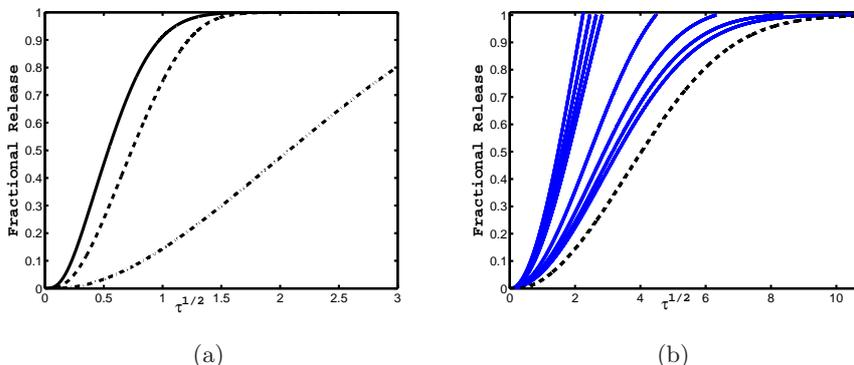
Figure 6: Fractional release profiles. In (a) the dependence of the release pattern on the solubility. The solid, dashed and dotted-dashed correspond to  $c_s/m_0 = 1.5, 0.5, 0.05$  respectively. In (b) the effect of erosion on dissolution is shown. The dashed line correspond to dissolution only. The dark solid lines from left to right are release profiles with increasing value of erosion velocity.
