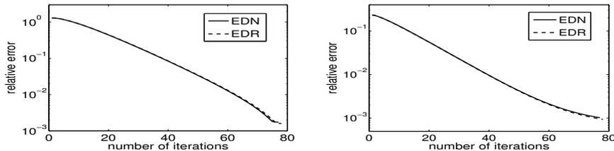
Figure 8: Relative errors in  $L^\infty$  norm with optimal relaxation parameter. Left: fluid velocity error, right: structure displacement error -  $t = 0.004$  s.
