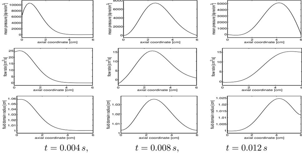
Figure 3: ERN scheme. Mean pressure (top), flow rate (middle) and fluid domain radius (bottom) at three time instants.
