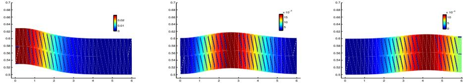
Figure 4: Displacement of the structure - ERN scheme -  $t = 0.004 s$  (left),  $t = 0.008 s$  (middle) and at  $t = 0.012 s$  (right).
