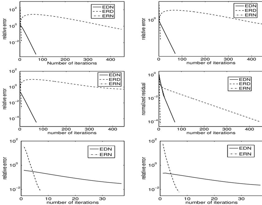
Figure 5: Relative errors in  $L^\infty$  norm with optimal relaxation parameter. Top, left: fluid velocity error,  $t = 0.004$  s. Top, right: pressure error,  $t = 0.004$  s. Middle, left: structure displacement error,  $t = 0.004$  s. Middle, right: residual normalized with the initial one,  $t = 0.004$  s. Bottom, left: fluid velocity error,  $t = 0.012$  s. Bottom, right: structure displacement error,  $t = 0.012$  s.
