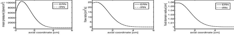
Figure 6: Comparison between the ERN and IRN solutions. Mean pressure (left), flow rate (middle) and fluid domain radius (right) -  $t = 0.004$  s.
