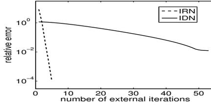
Figure 7: Relative errors in  $L^\infty$  norm with optimal relaxation parameter for IDN and IRN: fluid velocity error -  $t = 0.004$  s.
