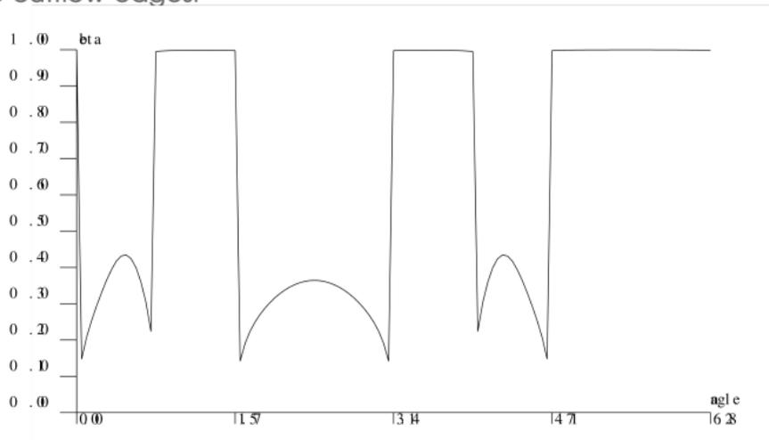
Values of the inf-sup constant  $\beta_h$  for the rotated unit triangle of order  $p = 2$ ,  $b = (1, 0)$ ,  $c = 1$ , and test space consisting of polynomials of order  $p + 1$ .
