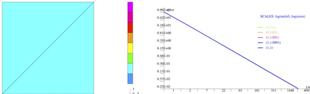
Left: initial mesh. Right:  $h$ -convergence results for a smooth exact solution and  $b = (1, 1.1), (1, 1.01), (1, 1.001), (1, 1.0001), (1, 1)$ .
