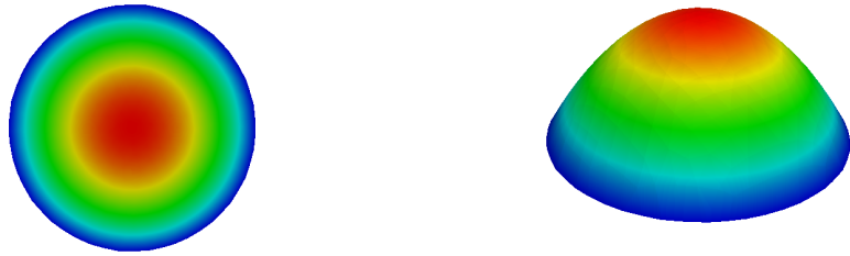
Figure 4.2: Adimensional images of the velocity field (left) and of the shape of the parabolic velocity profile (right) at the inlet for the cylindrical case.
