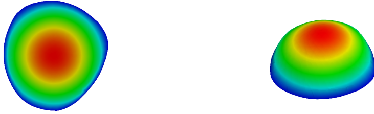
Figure 4.6: Adimensional images of the velocity field (left) and the shape of the parabolic profile for the velocity (right) at the inlet for the Stenotic case.
