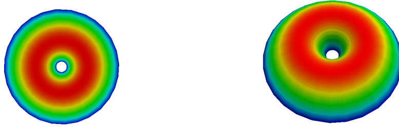
Figure 4.4: Adimensional images of the velocity field (left) and the shape of the parabolic profile for the velocity (right) at the inlet for the cylindrical perforated case.
