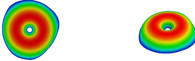
Figure 4.8: Adimensional images of the velocity field (left) and of the shape of the parabolic profile (right) for the velocity at the inlet for the Stenotic pwg case.
