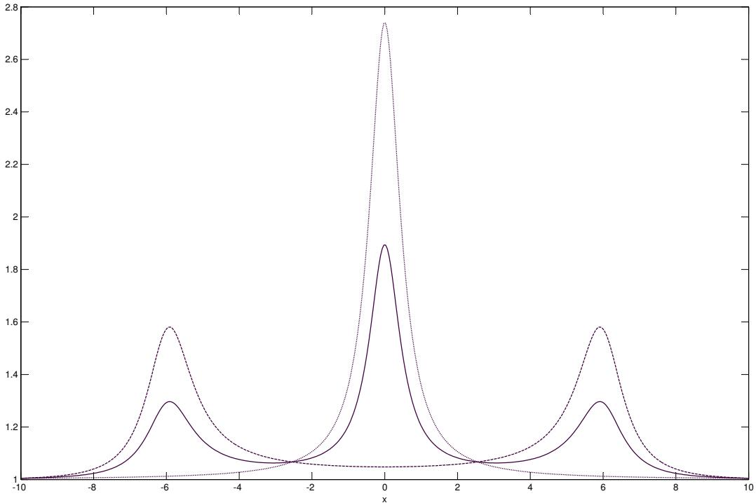
Figure 3: Formation of the Mollow triplet. The parameters are  $\gamma = 1$ ,  $k_0 = \bar{n} = 0$ ,  $|\alpha_1|^2 = |\alpha_2|^2 = 0.45$ ,  $k_1 = 0.0$ ,  $\Delta\omega = 0.0$ ,  $\Omega = 6.0$  and: (dashed line)  $\vartheta_2 = 0.0$ ; (solid line)  $\vartheta_2 = \frac{\pi}{4}$ ; (dotted line)  $\vartheta_2 = \frac{\pi}{2}$ .
