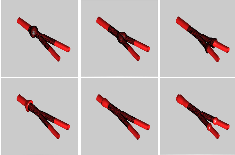
Figure 13: (from [36]). Snapshots of the simulation of a vascular bifurcation with a prosthesis, carried out with a 1D model. The three pictures in the top row illustrate the case of a prosthesis softer than the arterial wall. The most relevant reflection is at the distal interface between the prosthesis and the vessels (right). At the bottom row the results obtained using the same boundary data but with a prosthesis stiffer than the vascular wall. The most relevant reflection is at the proximal interface between the vessel and the prosthesis (left) and it back propagates up to the heart.
