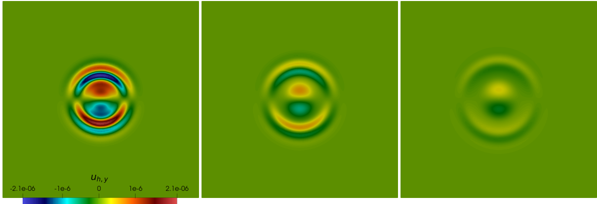
Figure 5: Wave propagation in poroelastic medium: computed vertical component of the velocity u_{h,y} at the time instants t = 0.8s (left), t = 0.9s (center), t = 1s (right).
