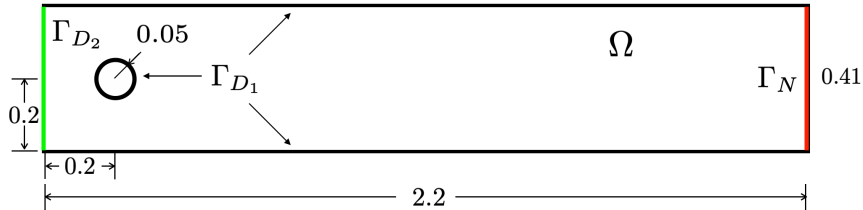
Figure 11: Test 4 : geometrical configuration, domain and boundaries.
