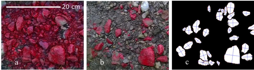
Figure (11) (a) Red pebbles painted before an event, (b) post-event image of the same area; (c) estimation of the dimensions of the remaining pebbles
