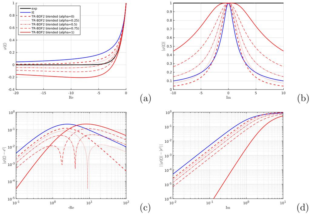
Figure 1: Hybrid TR-BDF2 in comparison with implicit Euler: *a*) stability functions along the negative real axis, *b*) modulus of the stability functions along the imaginary axis, *c*) absolute error functions along the negative real axis showing the asymptotic and non-asymptotic ranges, *d*) absolute error functions along the positive imaginary axis.
