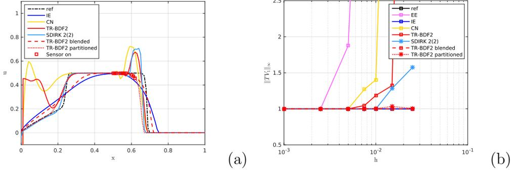
Figure 11: Buckley-Leverett equation with Koren limiter and non smooth initial condition: *a)* solution at final time  $t = 0.125$  when using  $h = 0.025$ , *b)*  $TV$ -space  $l^\infty$ -time seminorm.
