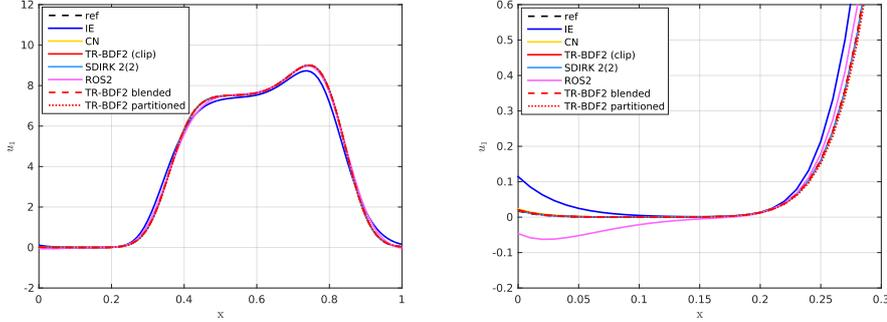
Figure 7: Advection diffusion reaction problem with non smooth initial condition: *a*) solution for  $u_1(t = T)$  when using  $h = 0.100$ , *b*) close-up in the region of positivity violation from ROS2.
