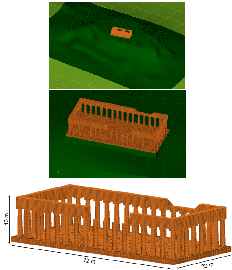
Fig. 4: 3D computational meshes of the Acropolis hill and the Parthenon.
