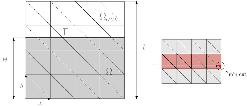
Figure 6: The geometry and triangulation of the computational domain used for Test 1 is shown on the left. On the right, a zoom at the intersection of the level set curve and the triangulation illustrates how small cut-elements appear.
