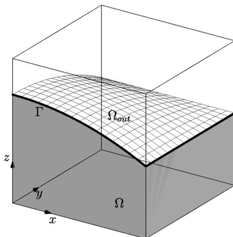
Figure 1: A sketch of the domain. The dark gray zone is the physical domain ( $\Omega$ ) while the white zone is the fictitious region ( $\Omega_{out}$ ). The interface between the physical and the fictitious regions is the surface  $\Gamma$ .
