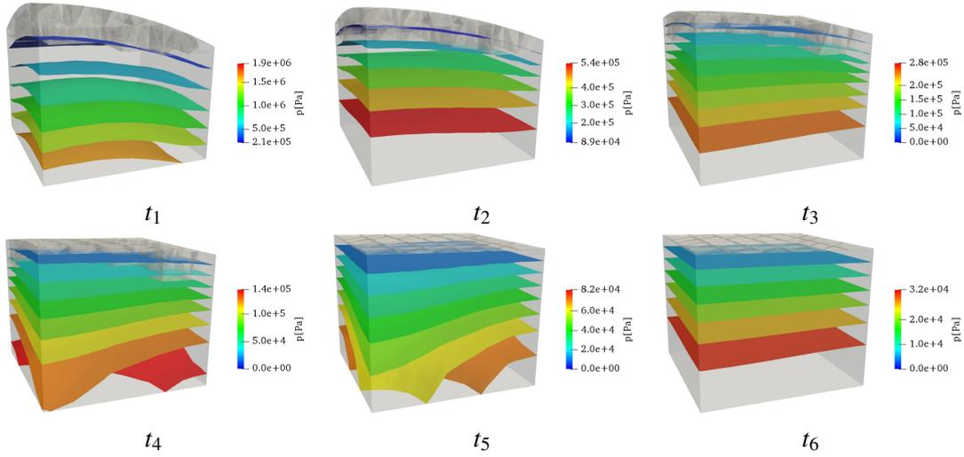
Figure 9: Pressure field at different time steps for Test 2.
