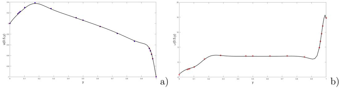
Figure 6: Lid driven cavity benchmark at  $Re = 1000$ , adaptive simulation: a)  $u$  velocity component values along the middle of the cavity, b)  $\omega$  values along the middle of the cavity. The continuous line denotes the numerical solution and the dots the reference solution values from [15].
