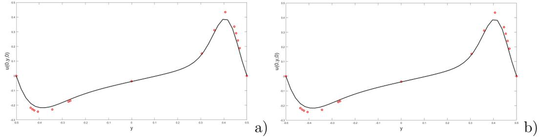
Figure 11: 3D lid driven cavity benchmark at  $Re = 1000$ , a)  $u$  velocity component values along the  $y$  axis for adaptive mesh simulation, b)  $u$  velocity component values along the  $y$  axis for fixed grid simulation. The continuous line denotes the numerical solution and the dots the reference solution values from [1].
