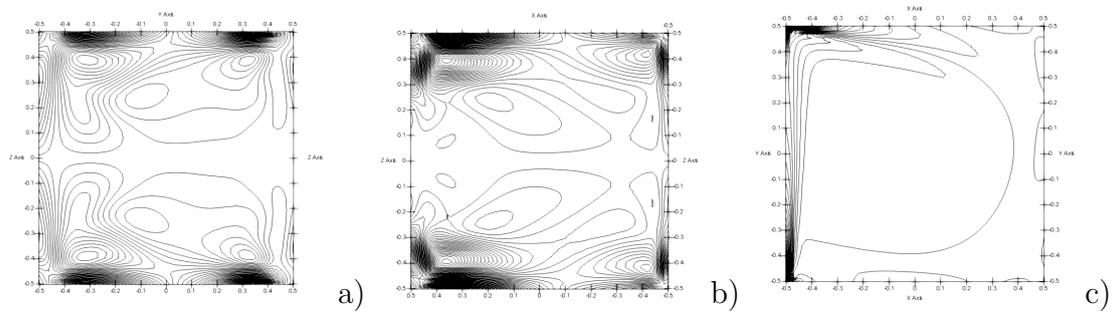
Figure 10: 3D lid driven cavity benchmark at  $Re = 1000$ , a) Vorticity ( $\omega_x$ ) contours at  $x = 0$ , b) Vorticity ( $\omega_y$ ) contours at  $y = 0$ , Vorticity ( $\omega_z$ ) contours at  $z = 0$
