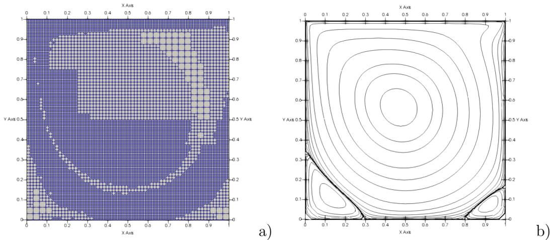
Figure 5: Lid driven cavity benchmark at  $Re = 1000$ , adaptive simulation: a) final mesh after adaptive refinement, b) streamfunction contours. Contour values as in [16].
