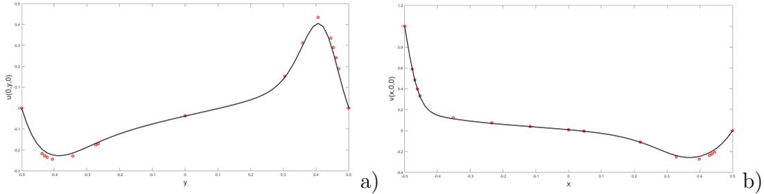
Figure 8: 3D lid driven cavity benchmark at  $Re = 1000$ , fixed mesh simulation with  $N_e =$  elements in each coordinate directions, a)  $v$  velocity component values along the  $x$  axis b)  $u$  velocity component values along the  $y$  axis. The continuous line denotes the numerical solution and the dots the reference solution values from [1].
