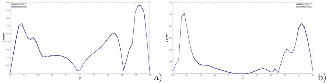
Figure 13: 3D lid driven cavity benchmark at  $Re = 1000$ , a)  $u$  velocity component component for the plane  $x = 0, z = 0$  with reference solution values from [1] interpolated, b)  $v$  velocity component comparison for the plane  $y = 0, z = 0$  with reference solution values from [1] interpolated. The continuous black line denotes the result with fixed mesh, the blue one denotes the results with adaptive mesh refinement.
