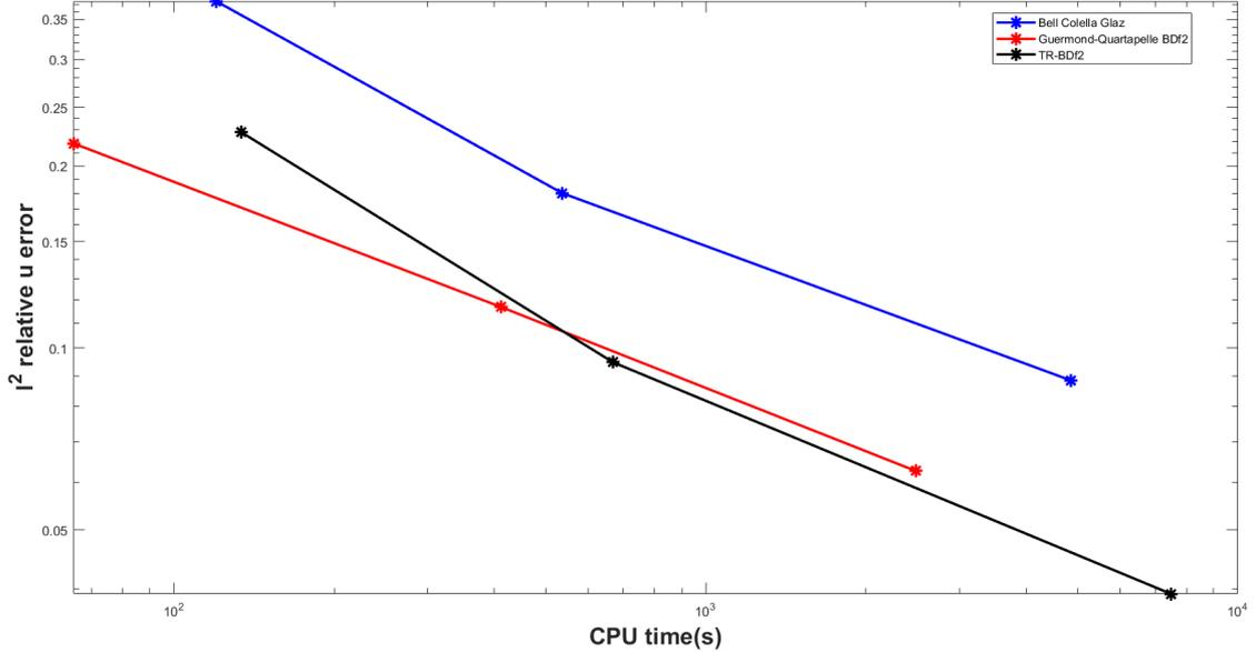
Figure 4: Lid driven cavity benchmark at  $Re = 1000$ ,  $l^2$  relative errors with respect to the reference solution values from [15] interpolated along the middle. The continuous black line denotes the result with the proposed method, the red one the results of [33] and the blue dots the results of [10].
