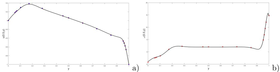
Figure 2: Lid driven cavity benchmark at  $Re = 1000$ : a)  $u$  velocity component values along the middle of the cavity, b)  $\omega$  values along the middle of the cavity. The continuous line denotes the numerical solution and the dots the reference solution values from [15].
