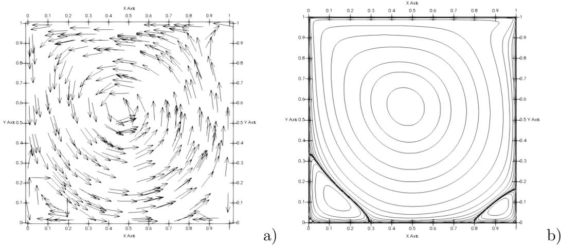
Figure 1: Lid driven cavity benchmark at  $Re = 1000$ : a) flow field, b) streamfunction contours. Contour values are chosen as in [16].
