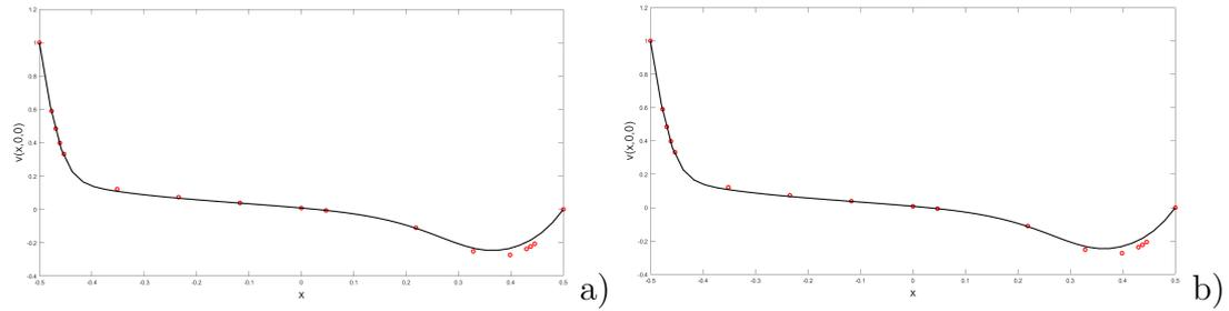
Figure 12: 3D lid driven cavity benchmark at  $Re = 1000$ , a)  $v$  velocity component values along the  $x$  axis for adaptive mesh simulation, b)  $v$  velocity component values along the  $x$  axis for fixed grid simulation. The continuous line denotes the numerical solution and the dots the reference solution values from [1].
