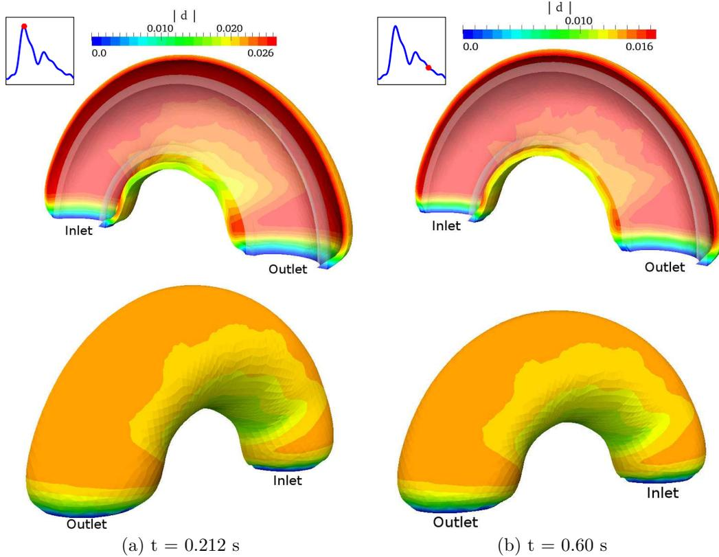
Figure 19: Magnitude of the vessel wall displacement  $\hat{d}$  [cm] in the deformed fluid domain. Constitutive model for the arterial wall: EXP2. In the first row, the gray overlay represents the undeformed domain
