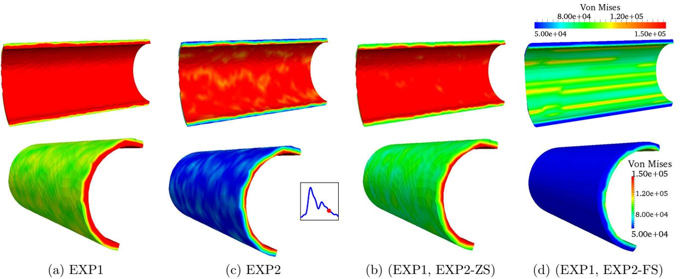
Figure 16: Von Mises stress [dyn/cm<sup>2</sup>] for the different constitutive models at the time  $t = 0.600$  s. Internal view (top); external view (bottom).
