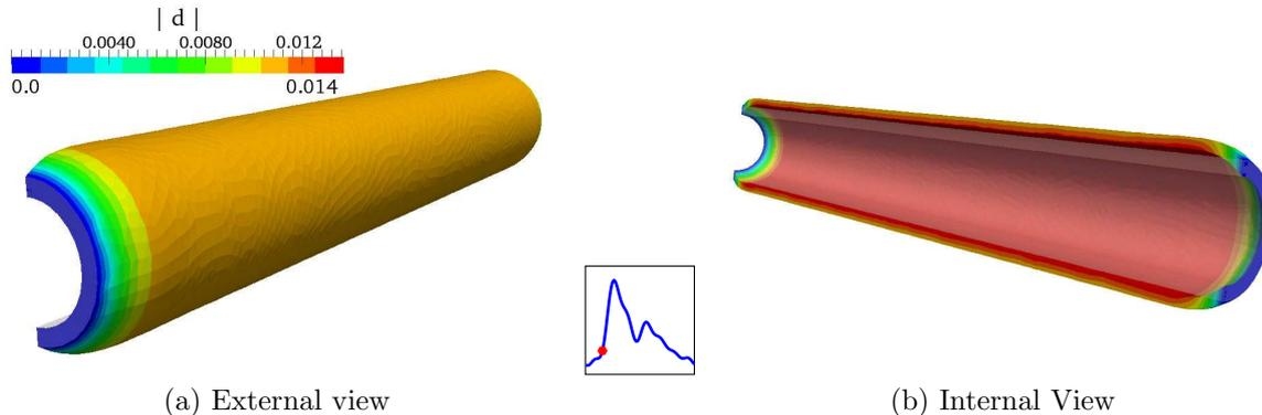
Figure 8: Displacement magnitude [cm] on the deformed vessel wall. (a) External view; (b) internal view. Time  $t = 0.100$  s. Constitutive model EXP2. The gray overlay represents the undeformed domain
