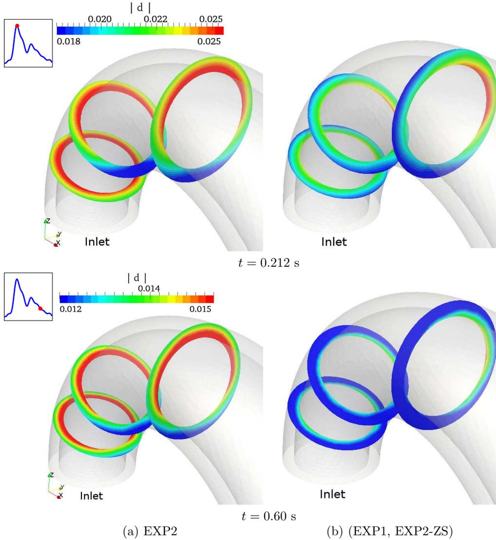
Figure 21: Magnitude of the vessel wall displacement  $\hat{d}$  [cm] on three different radial sections of the vessel wall for the EXP2 and (EXP1, EXP2-ZS) models at different times along the heart beat
