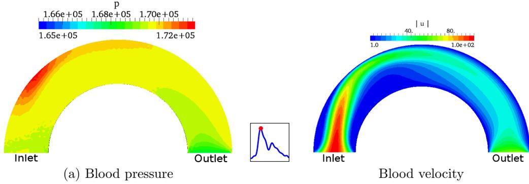
Figure 18: Blood pressure  $p$  [dyn/cm<sup>2</sup>] and velocity [cm/s] in the undeformed fluid domain at the time  $t = 0.212$  s. Constitutive model for the arterial wall: EXP2
