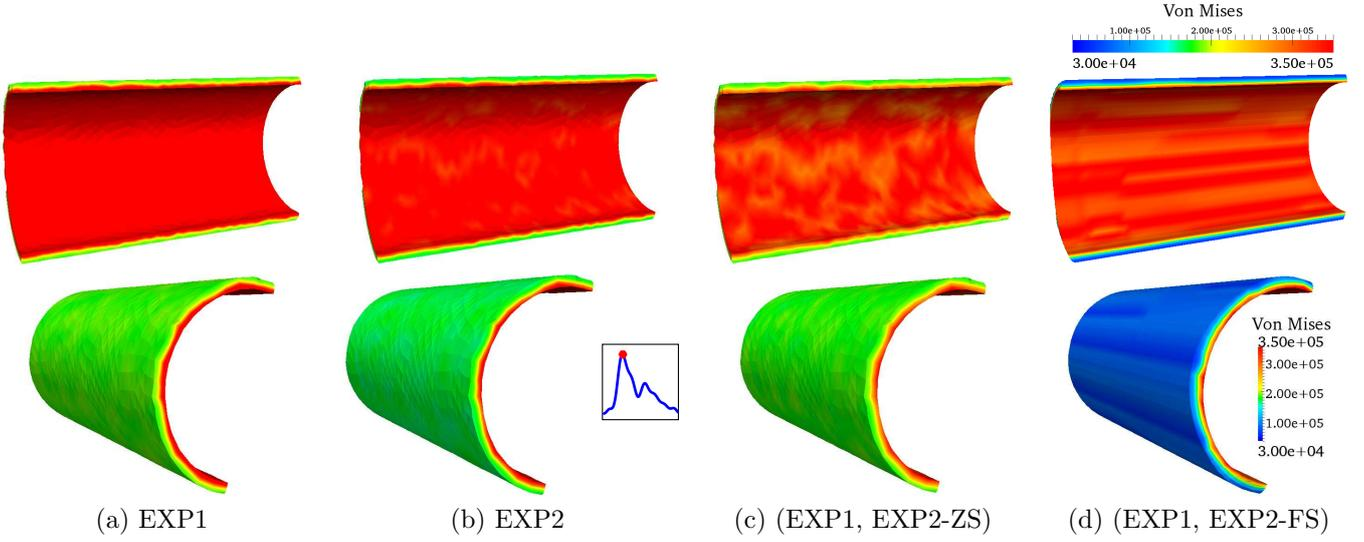
Figure 15: Von Mises stress [dyn/cm<sup>2</sup>] for the different constitutive models at the time  $t = 0.212$  s. Internal view (top); external view (bottom)
