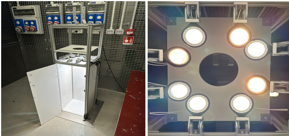
Figure 1: Light box used for hyperspectral image collection.
