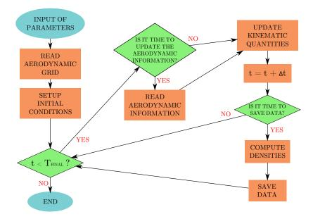
Figure 2: Flow chart of the serial program.
