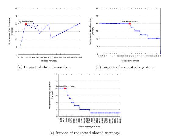
Figure 4: Impact of parameters variations on the occupancy of the SMs.
