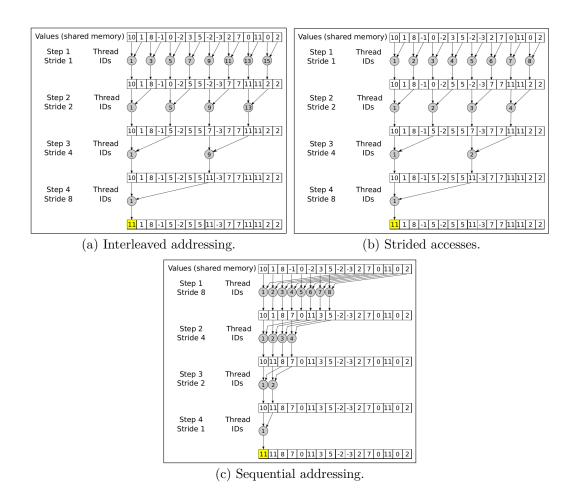
Figure 3: Different implementations of the parallel reduction of a 1D array.
