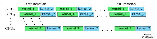
Figure 6: Kernel execution is a non-blocking CUDA function.
