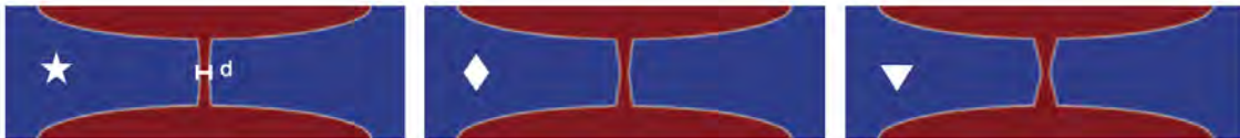
Figure 16: Dissolution of the conductive filament in a cation-based RRAM device: different initial configurations of the CF. Each configuration is associated with a different marker.
