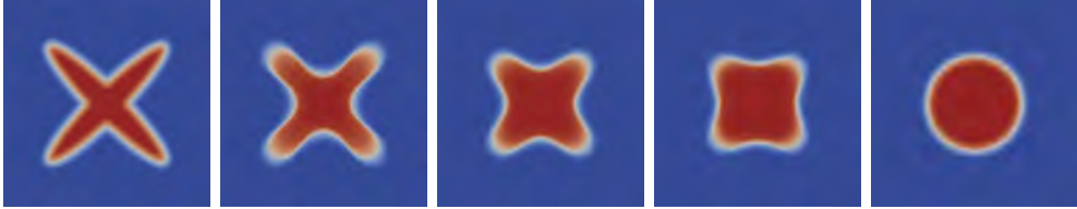
Figure 7: Evolution of a star into a circle under the effect of the surface diffusion due to curvature gradient: t = 0s, 0.1s, 0.3s, 0.4s, 1s (from left to right).
