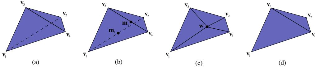
Figure 2: Procedure in the case of sliver. In (d) the faces that could remain in the tetrahedral mesh.
