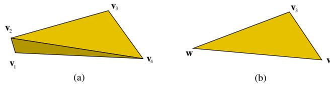
Figure 4: Procedure in the case of wedge. In (b) the faces that could remain in the tetrahedral mesh.
