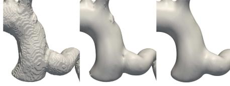
Figure 7: Polygonal surface mesh: result of the marching cube method (left), Gaussian filters (center), and Taubin algorithm (right). Posterior views.
