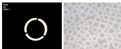
Figure 10: Trilobe die. Die Geometry (left) and extruded polymer profiles (right). (Courtesy of RadiciYarn S.p.A.).
