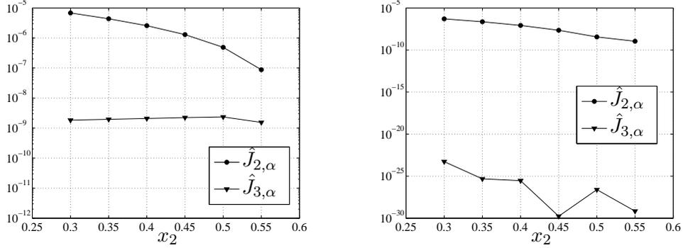
Figure 8: The minimum values  $\hat{J}_{2,\alpha}$  and  $\hat{J}_{3,\alpha}$  versus the size of the overlap, obtained with  $\nu = 0.1$ ,  $b = 1$  at left and  $\nu = 0.01$ ,  $b = -1$  at right. For both cases  $\alpha = 0$ , we have decomposed  $\Omega$  in 20 equal spectral elements of equal size  $H = 0.5$  and  $N = 4$  in each element,  $\Omega_1 = (0, 0.6)$  and  $\Omega_2 = (x_2, 1)$ . The size of the overlap is  $meas(\Omega_{12}) = 0.6 - x_2$ .
