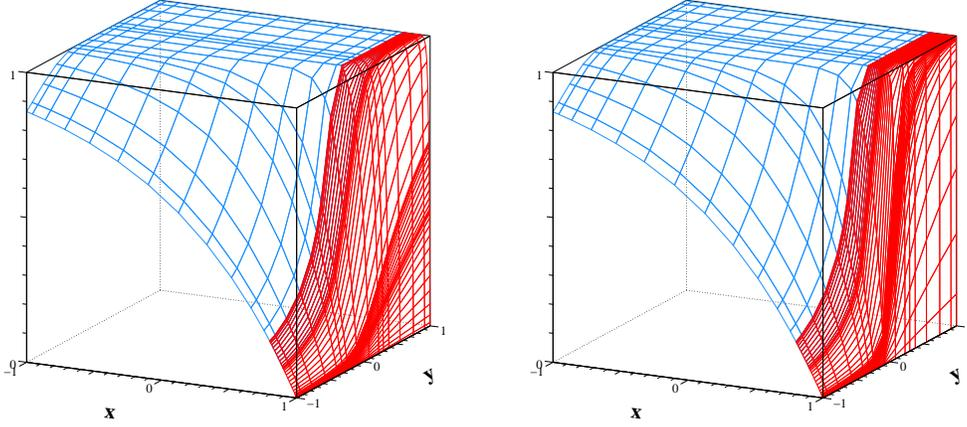
Figure 10: Test case #1. Numerical solution for  $\nu = 10^{-2}$  (left) and  $\nu = 10^{-3}$  (right) obtained through the 3-controls approach with  $\alpha = 0$ . The overlap is  $\Omega_{12} = (.7, .8) \times (-1, 1)$ . The minimum values of the cost functional  $J$  are  $\hat{J}_{3,\alpha} = 1.97 \cdot 10^{-11}$  for  $\nu = 10^{-2}$  and  $\hat{J}_{3,\alpha} = 5.81 \cdot 10^{-11}$  for  $\nu = 10^{-3}$ .
