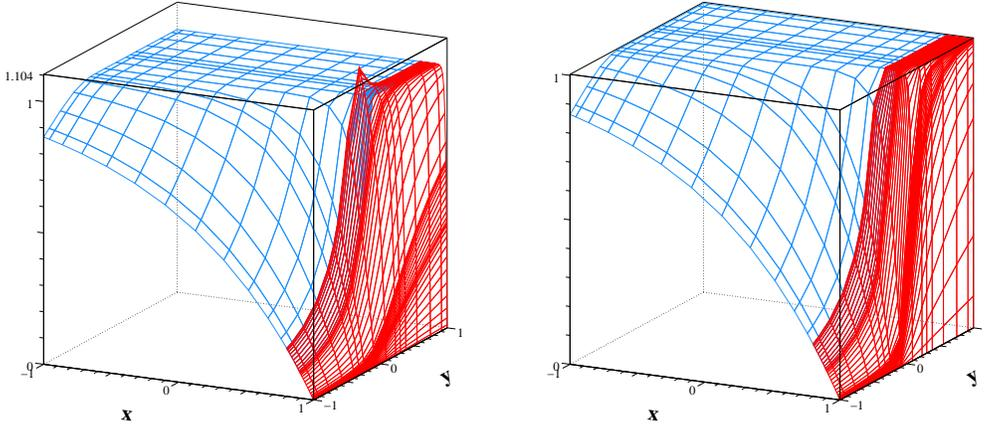
Figure 9: Test case #1. Numerical solution for  $\nu = 10^{-2}$  (left) and  $\nu = 10^{-3}$  (right) obtained through the 2-controls approach with  $\alpha = 0$ . The overlap is  $\Omega_{12} = (.7, .8) \times (-1, 1)$ . The minimum values of the cost functional  $J$  are  $\hat{J}_{2,\alpha} = 5.67 \cdot 10^{-5}$  for  $\nu = 10^{-2}$  and  $\hat{J}_{2,\alpha} = 4.92 \cdot 10^{-7}$  for  $\nu = 10^{-3}$ .
