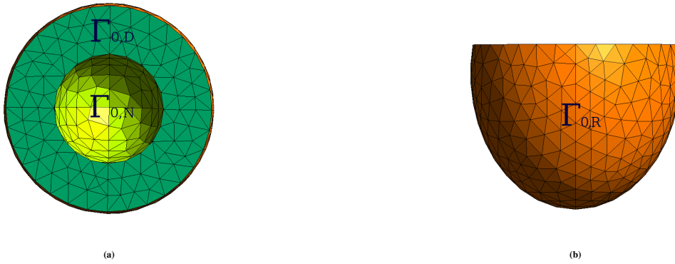
FIGURE 1 Idealized left ventricular geometry with boundaries \Gamma_{0,D} , \Gamma_{0,N} , \Gamma_{0,R} highlighted in different colors to distinguish the three subsets of \partial\Omega_0 on which we set the boundary conditions (Dirichlet, Natural and Robin, respectively).
