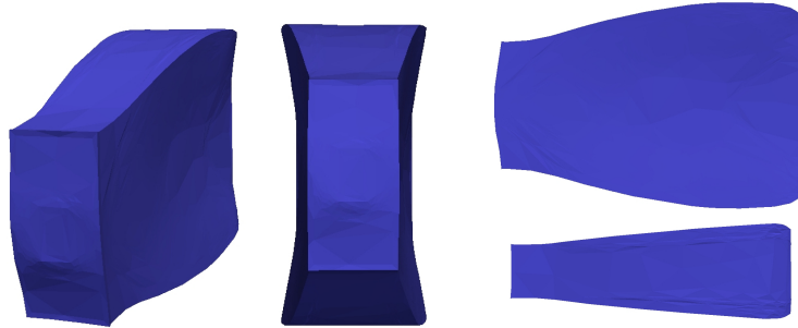
Figure 4: The cantilever test case (SO): optimized structure (left), lateral (center), frontal (top-right) and top (bottom-right) views of the optimized structure.
