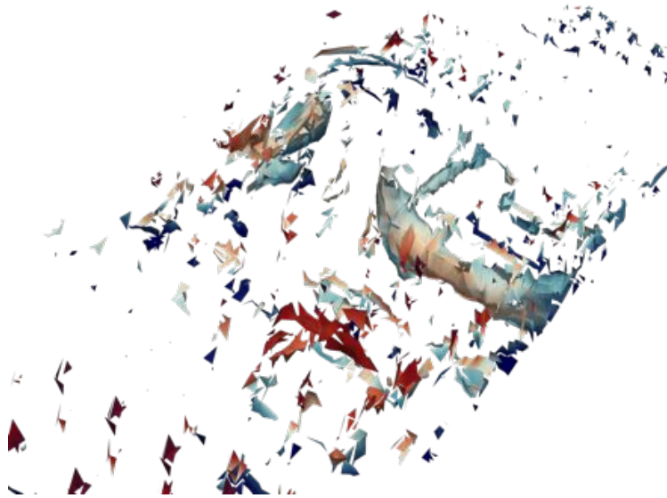
Figure 9: Isosurfaces at t = 4 for Re = 6000 (Smagorinsky model LES) (a) density isosurfaces ( \rho = 0.72, 0.82, 0.85, 0.88, 0.98 ). (b) Q = 20 isosurface (colored by density).
