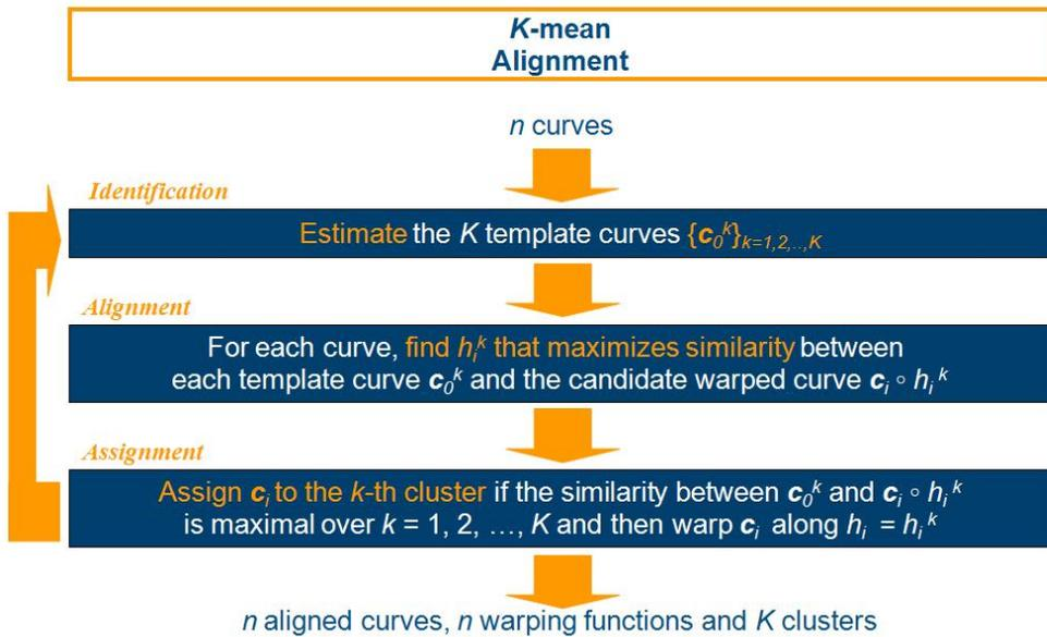
Figure 2: Schematic flowchart of the  $k$ -mean alignment algorithm. Index  $i$  refers to the sample unit while index  $k$  to the cluster.
