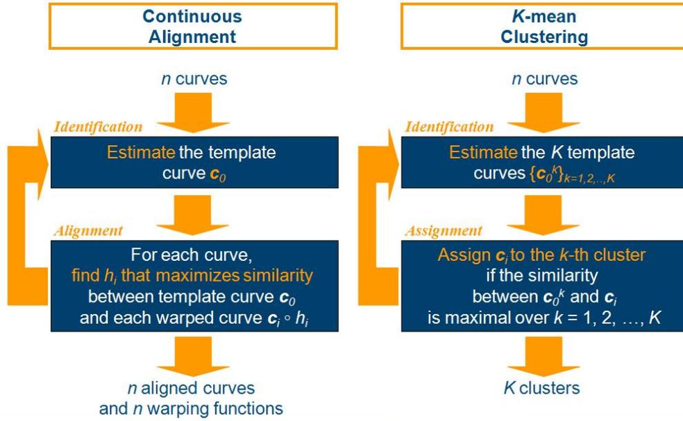
Figure 1: Schematic flowcharts of the Procrustes continuous registration algorithm (left) and the functional  $k$ -mean clustering algorithm (right). Index  $i$  refers to the sample unit while index  $k$  to the cluster.
